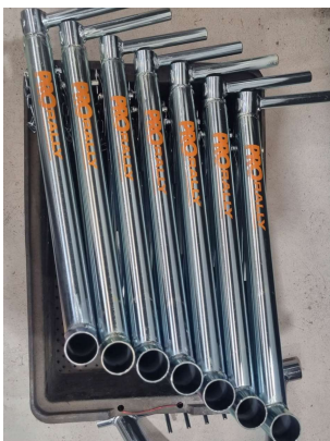
Adjustable Sill Stands designed and manufactured in-house at Pro Rally Motorsport
